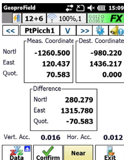
Figure 169: Vue Implantation (Stakeout)
